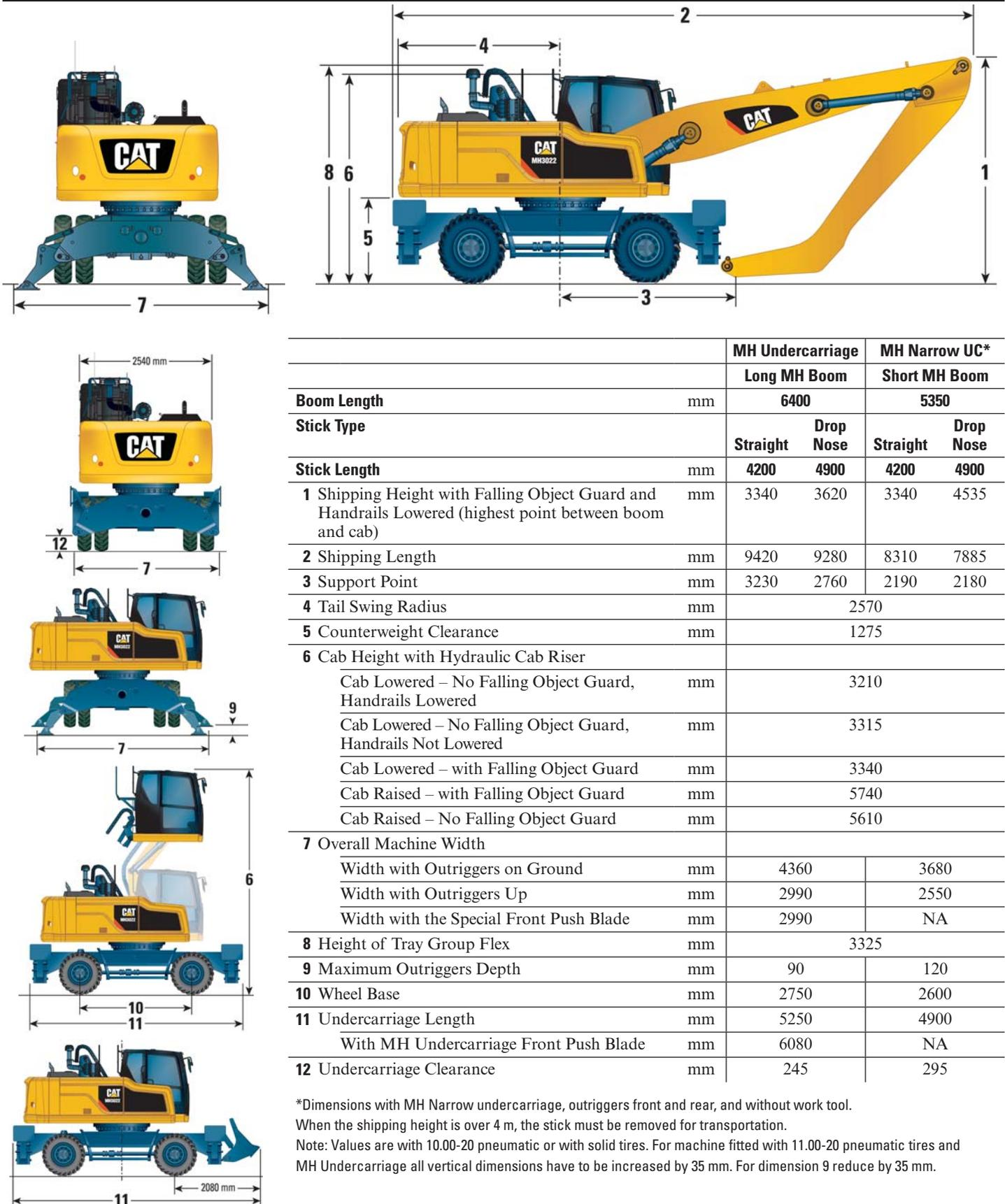
\*Dimensions with MH Narrow undercarriage, outriggers front and rear, and without work tool.
